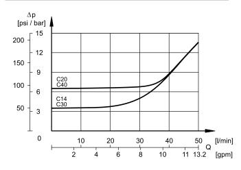
Pressure drops with flow  $A \rightarrow P$ . Obtained with  $Q_B = 0$  (de-energised coil - no current)
